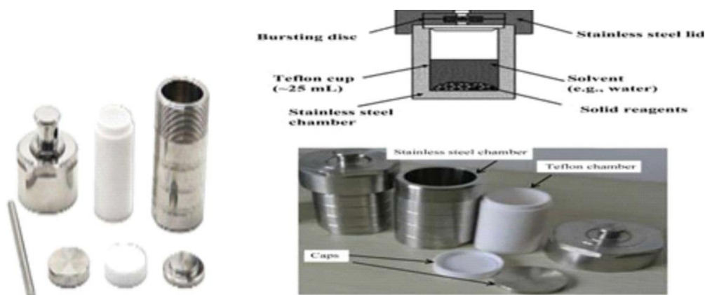
Fig.:Instrumentation required for hydrothermal method and auto-clave for hydro-thermal technique
